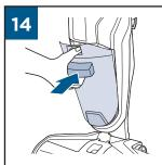
Angle the Dirty Water Tank back into body of machine inserting bottom first. Then tilt the top of the dirt tank toward the machine and push into place until you hear a "click".
