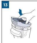
Once parts are dry, reassemble and replace the top of Dirty Water Tank.
