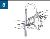
Rinse the float located at the bottom of the top of the Dirty Water Tank.
