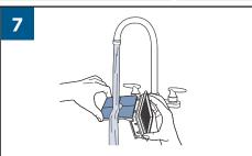
Hand wash the filter and screen with warm water and mild detergent.
