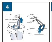
Remove strainer from Dirty Water Tank, then throw debris in trash.
