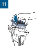
Place filter assembly back into the top of the Dirty Water Tank.
