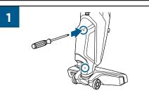
With a Phillips-head screwdriver, remove the 4 screws on the back of the unit. Then, lift off the back cover.
